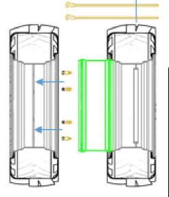
Install Eye bolts on your wheel centre and cut threaded hook rods to the required length.
