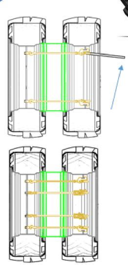
3.) Hook the threaded rods through the eyebolt and begin to install clamps. Use a pipe spanner to tighten.
